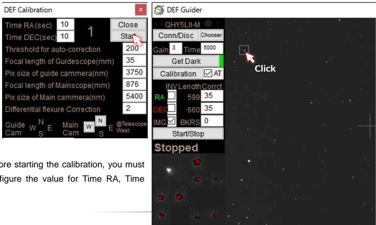
Before starting the calibration, you must configure the value for Time RA, Time
